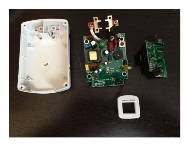
**Step #6**Replace these 5 capacitors using the provided kit.
